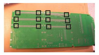
Not correct. Washers should be removed
